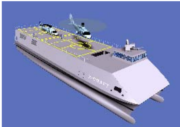
Titan X-Craft - Rolls Royce engines have been selected for X-Craft, an experimental high-speed aluminium catamaran.
