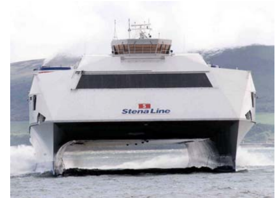
A catamaran is a type of boat consisting of two hulls joined by a frame. Catamarans were used as early as 5 th Century . (Picture shows the Rolls-Royce powered high speed ferry.)
