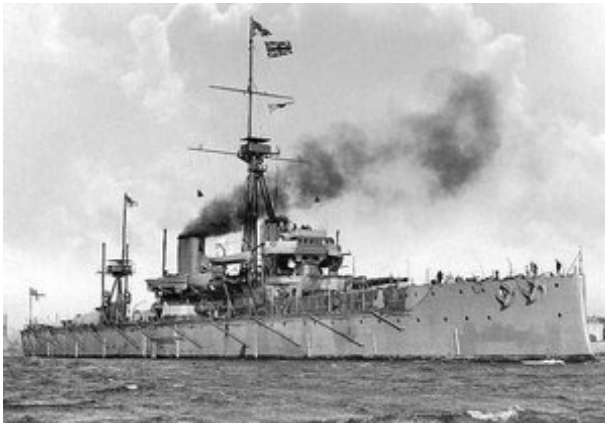
The sixth HMS Dreadnought of the British Royal Navy was the first battleship to be powered by steam turbines , making her the fastest warship of her size.
